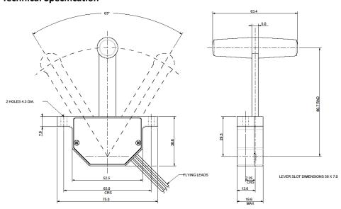
**Electrical** Mechanical Supply 5V ±0.5VDC Actuator travel 63° (±31.5° about centre) Typ. supply current 13.5mA Operating force 1.5N Max. supply current 10.0mA Weight 100g Overvoltage 24VDC **Expected life** 1 million operations -12VDC Reverse voltage protection Lever action Friction 10Ω 400mm Output impedance Lead length **Environmental Connections** -40°C to +50°C Colour Operating temperature Function -40°C to + 70°C Storage temperature Red +5VDC supply White Output Black 0V
